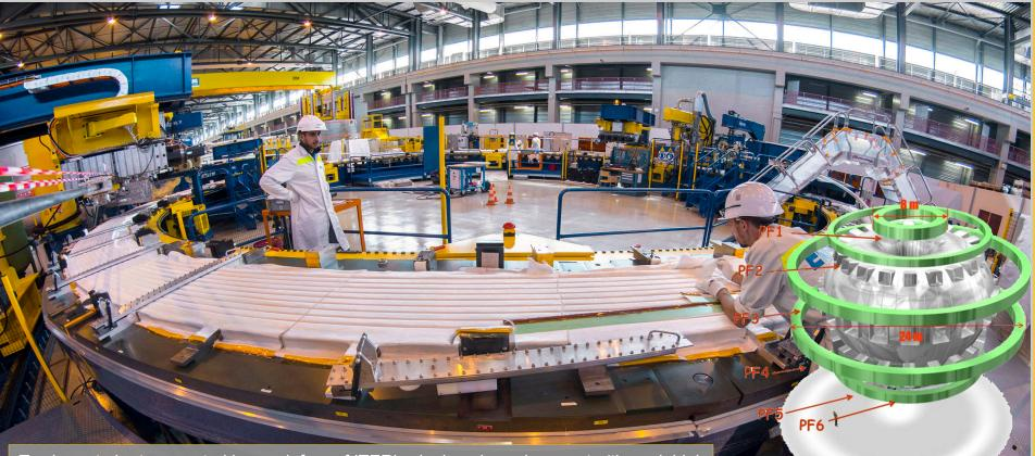
Too large to be transported by road, four of ITER's six ring-shaped magnets (the poloidal field coils, 8 to 24 m in diametre) will be assembled by Europe in this 12,000 m<sup>2</sup> facility.
