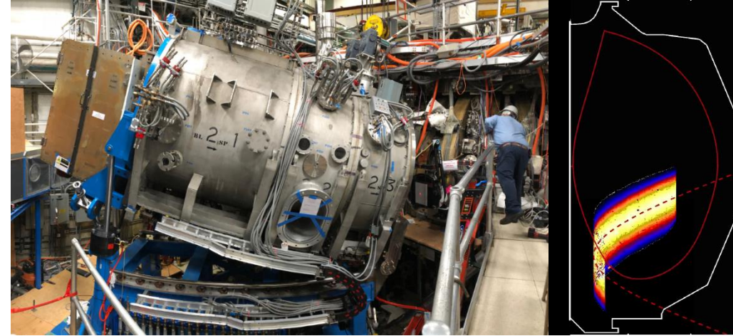
Off-axis neutral beam and imaging from beam-into-gas commissioning
