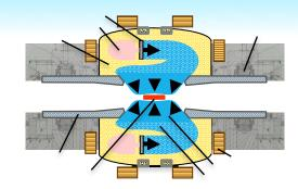
Piston-driven implosion of rotation-stabilized liquid metal liner to compress plasma. High shot rate for development system and multipurpose liner/blanket/thermal medium for power reactor.
