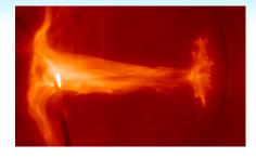
Collisions of plasma jets with targets in "reversed frame of reference" MIF analogue. Characterize dimensionality of adiabatic compression in MIF.
