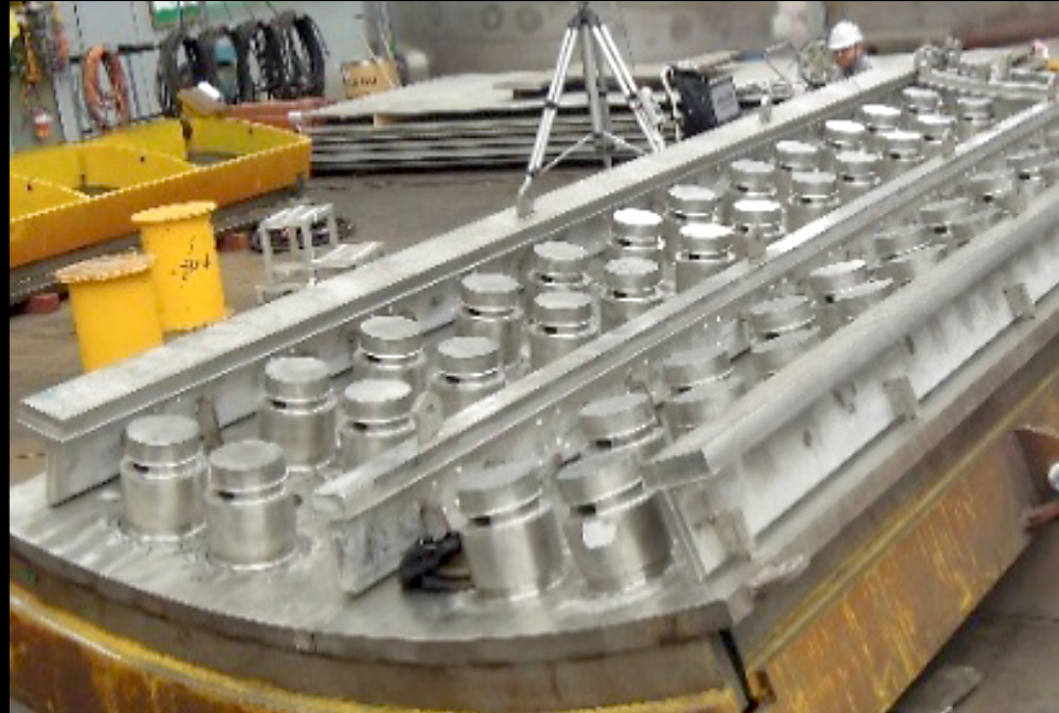
Vacuum vessel Sector 6 inner shell assembly, showing poloidal "t-ribs."
