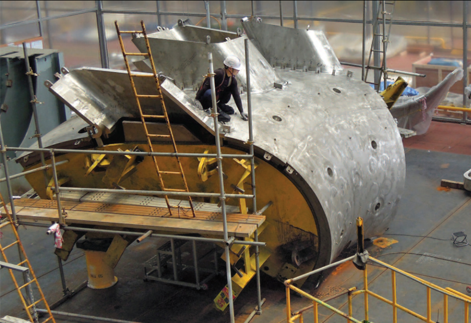
Port stub assembly for Sector 6 of the vacuum vessel.
