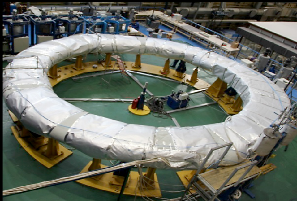
Vacuum pressure impregnation of a dummy poloidal field coil.
