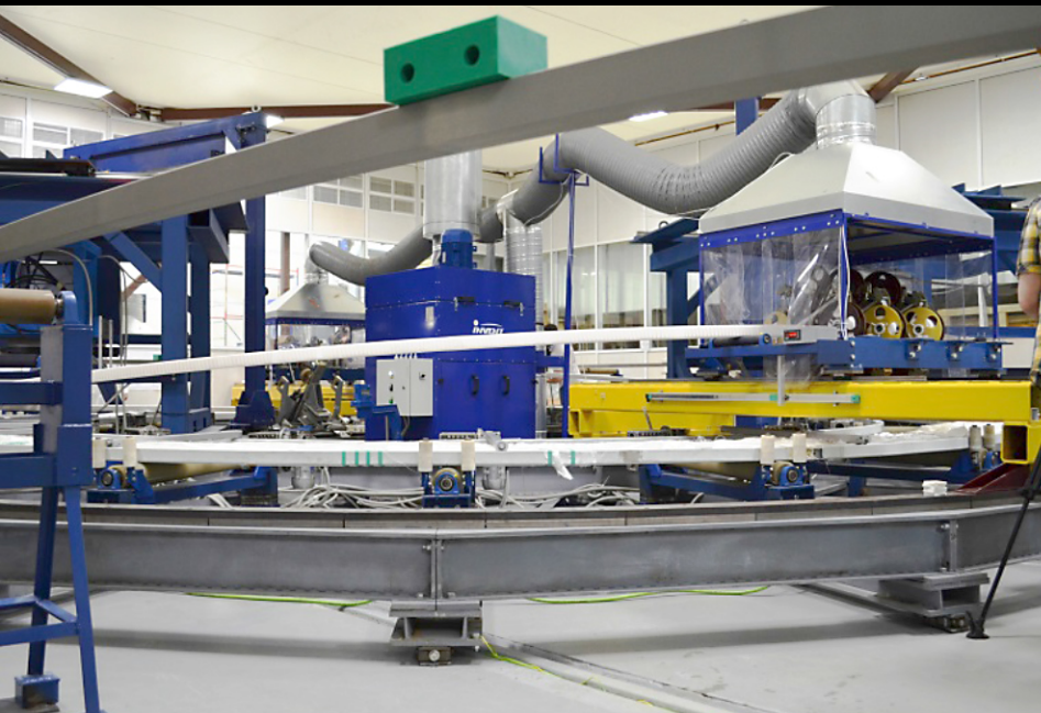
Winding of a double pancake for poloidal field coil 1.
