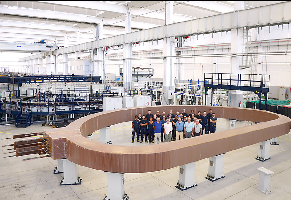
The first resin impregnated toroidal field coil winding pack was completed at ASG in La Spezia, Italy.
