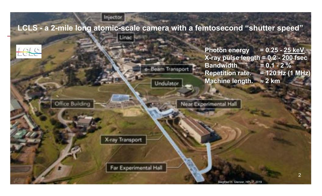
LCLS: coherent, extreme brightness x-rays (>109 increase over prior sources) resolving plasma waves and structure color
