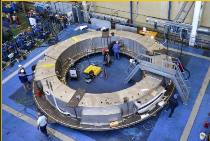
Poloidal field coil #1 is entering the final stages of fabrication in Saint Petersburg; FAT expected next month
