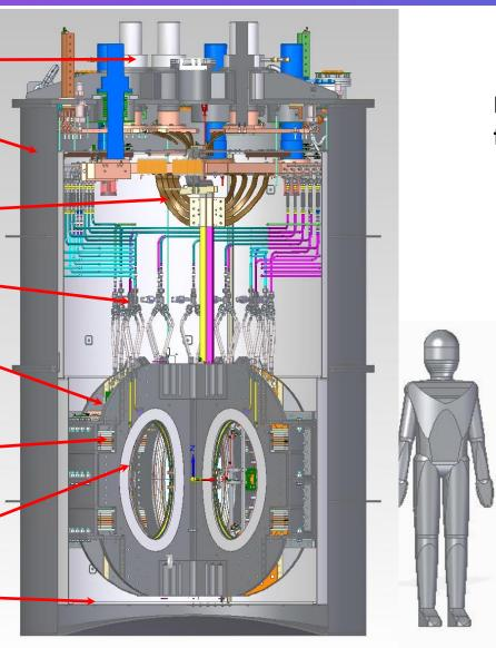
Demo4 is a conduction cooled, cryogen free, ~20 K HTS magnet test bed.
