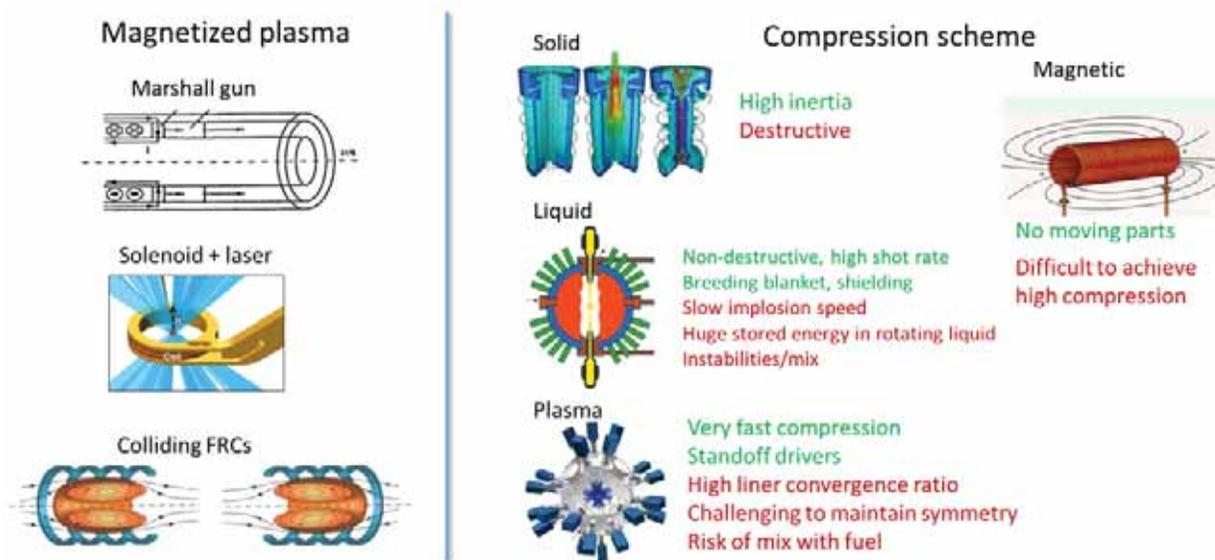
Figure 9. Ingredients of a MIF system. Many combinations of magnetized plasma and compression scheme are possible (though not all possibilities are practical). Only a subset of the plausible approaches has been tried.
