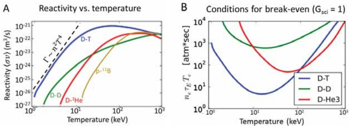
Figure 7. Thermodynamics of fusion reactions. A) Reactivity (reaction rate per particle) of the commonly studied fusion reactions. At temperatures  $< 100$  keV, the DT reaction is most favorable, but at temperatures  $> 100$  keV the  $p^{11}\text{B}$  reaction becomes comparable. B) Triple product to achieve scientific break-even as a function of temperature. For the DT reaction, the optimal temperature is 14 keV.
