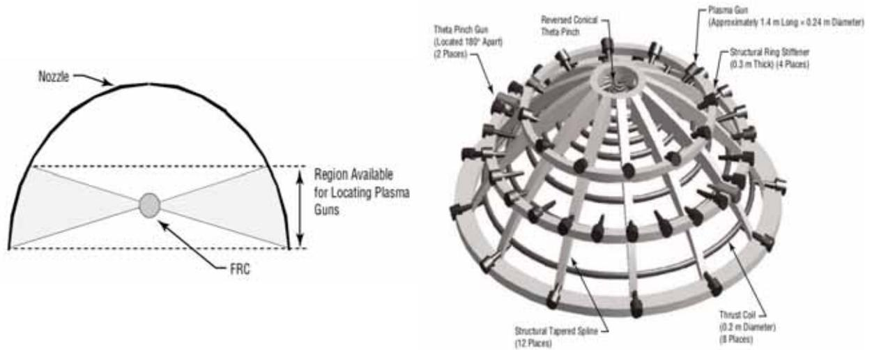
Figure 14. Distribution of plasma guns in the conceptual design of a fusion thruster. These guns inject DT plasma followed by an ordinary hydrogen ( $^1\text{H}$ ) “liner” to compress the fuel and also add to the propellant mass. The gray rings in the lower panel carry current to create a magnetic nozzle that deflects and expels the expanding exhaust gases.
