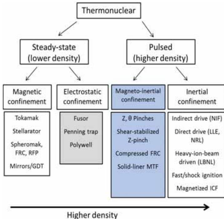
**Figure 4.** Approaches to controlled fusion. Thermonuclear approaches maintain an approximately Maxwell-Boltzmann velocity distribution, permitting each ion to undergo many Coulomb scattering events prior to a fusion reaction. MIF approaches are shaded in blue. Approaches unlikely to reach scientific break-even are shaded in grey. Image adapted from S. Hsu, LANL.
