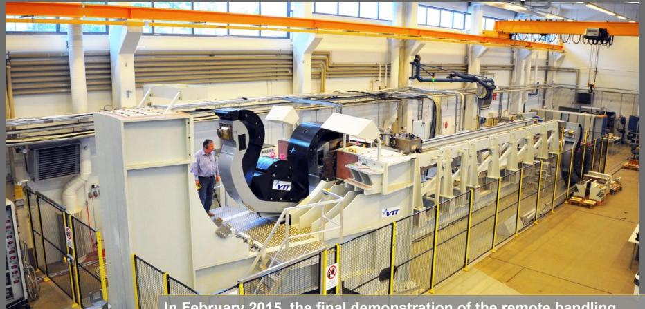
In February 2015, the final demonstration of the remote handling system for the divertor cassettes (an essential piece of the ITER Tokamak) was conducted at VTT Research Centre of the University of Tampere, Finland.
