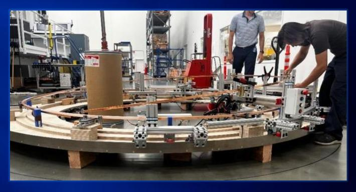
Demonstration of winding process for circular large bore and D-shaped coils in progress
