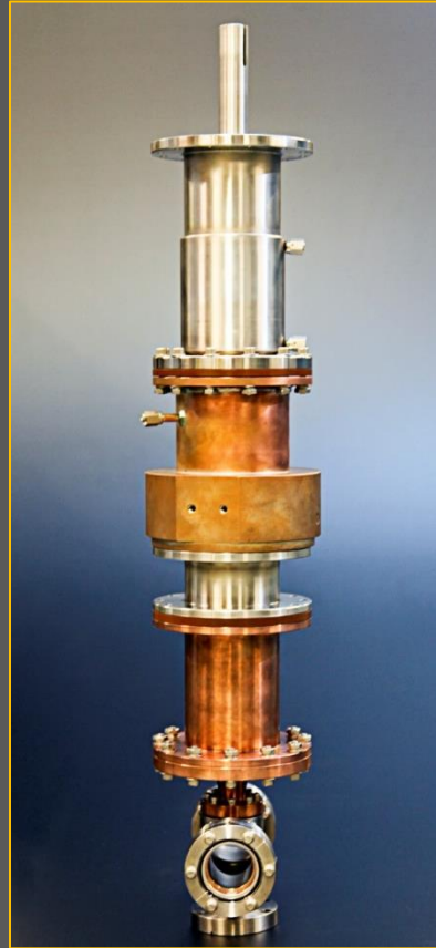
Twin screw pellet extruder developed at ORNL.
