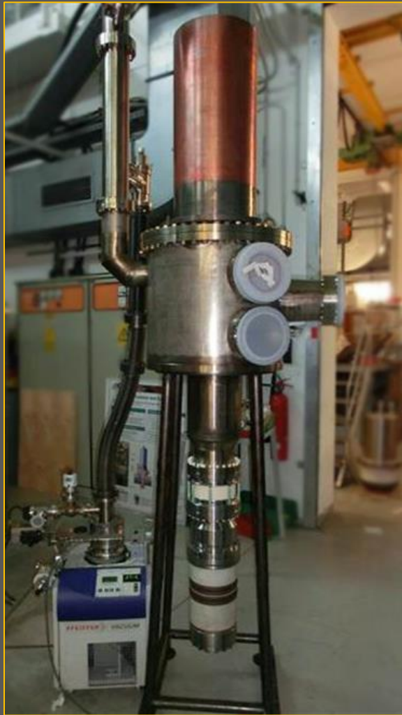
Gyrotron prototype developed by F4E (EU-DA).
