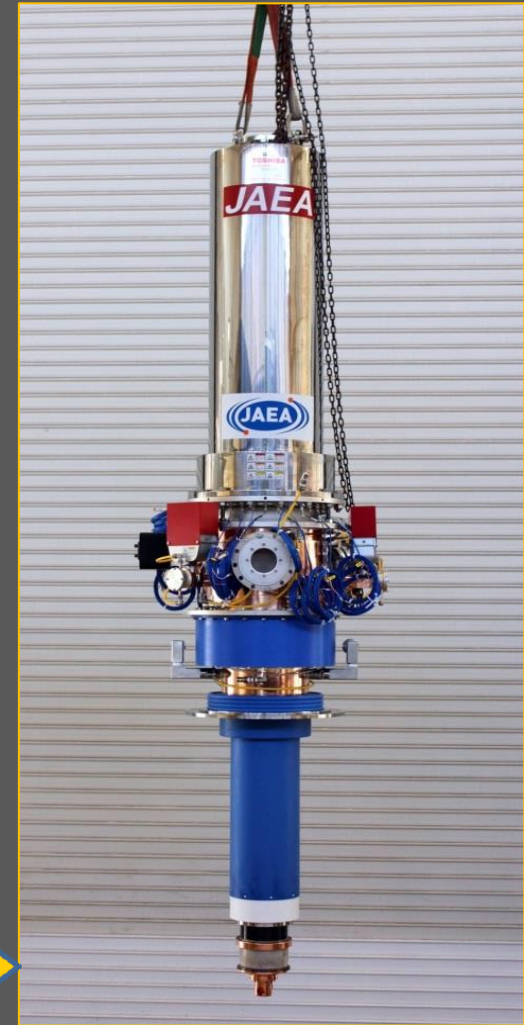
Gyrotron prototype developed by JA-DA.
