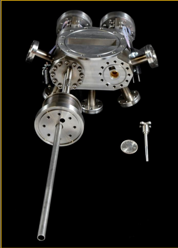
Dual nozzle prototype developed at ORNL (Oak Ridge National Laboratories, USA).
