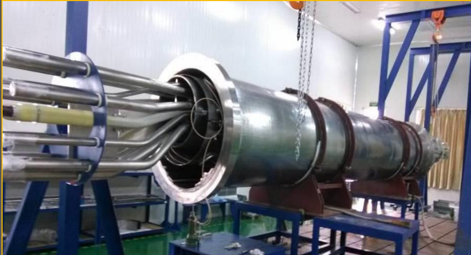
Internal components of a cryostat feeder prototype.
