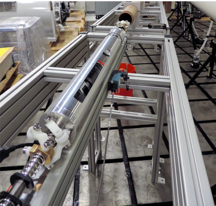
A laser-based wave guide inspection system was developed
