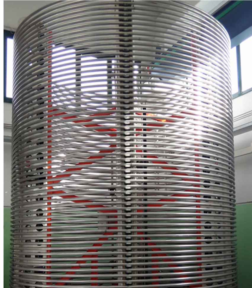
The conductor was jacketed and integrated at High Performance Magnetics in Tallahassee, FL and Criotec in Chivasso, Italy (above).
