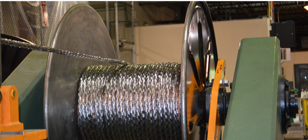
Cabling of the strand was performed by New England Wire Technologies in Lisbon, NH.
