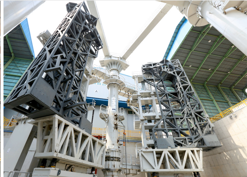
The first fully assembled, 800-tonne vacuum vessel sector sub-assembly tool (SSAT) has been test fitted and is ready to ship to the ITER site.
