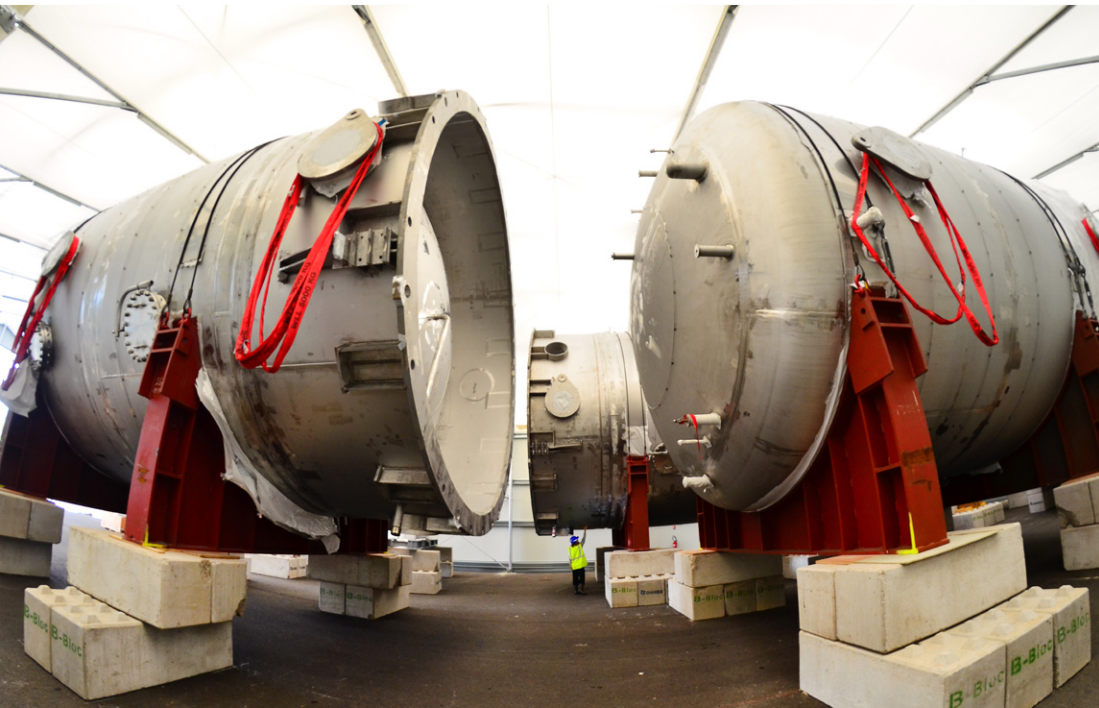
Drain tanks fabricated in the US were the first nuclear-certified components delivered to the ITER site (September 2015).
