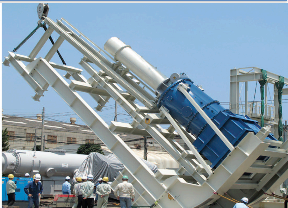
The 1 MV bushing at Hitachi for the full-scale ITER neutral beam injector. The bushing has since been delivered to the PRIMA neutral beam test facility in Italy for the MITICA (Megavolt ITER Injector and Concept Advancement) test bed. Photo: ITER Japan
