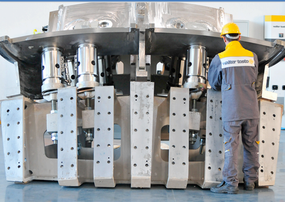
A poloidal segment of one vacuum vessel sector is fitted. Four segments, each weighing over 6 tonnes, form the full sector. Photo: Walter Tosto
