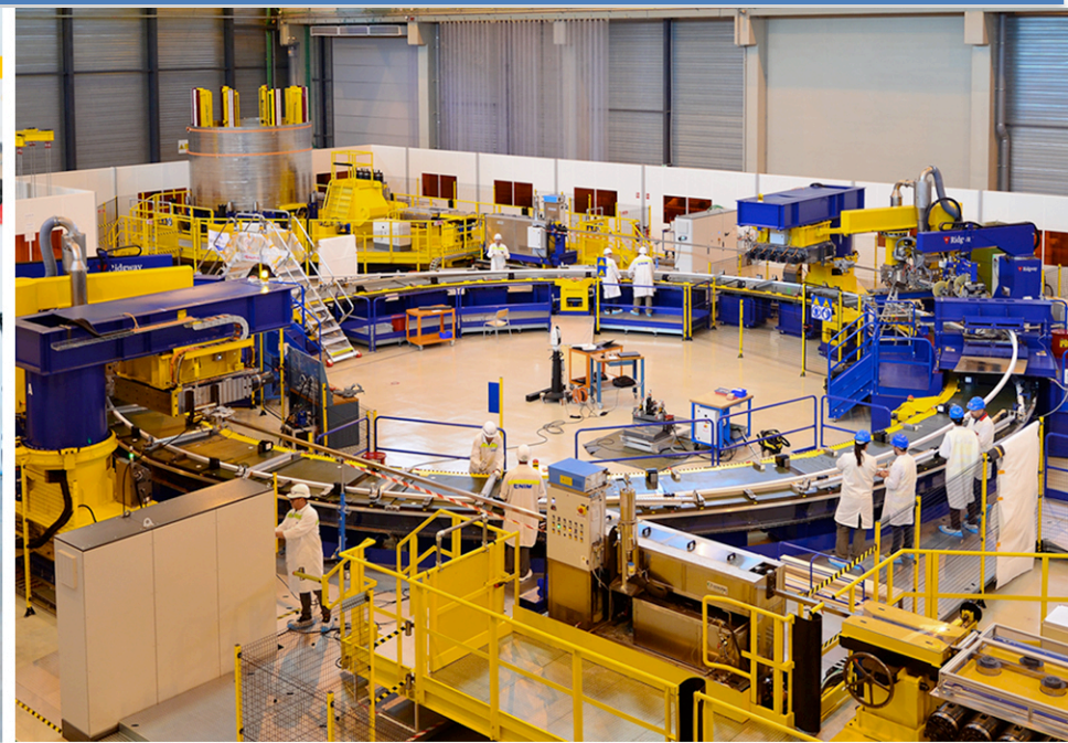
Production winding has begun for poloidal field #5. Photo: ITER Organization
